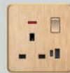
NS5563 15A 1 GANG SWITCHED SOCKET + 1 USB + 1 TYPE C + NEON DP 15A 250V~ 50/60Hz, 5V 2.1A
